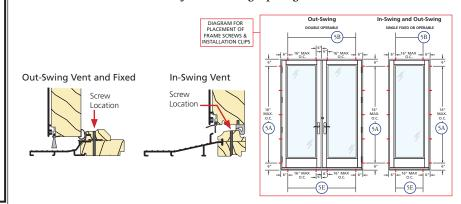
D. Secure the jambs and head of the door. Drive #10 x 3-1/2" corrosion resistant wood screws through the door frame and shim, into the rough framing. Drive the screws until snug but DO NOT overtighten the screws. DO NOT bend or bow the unit frame.
